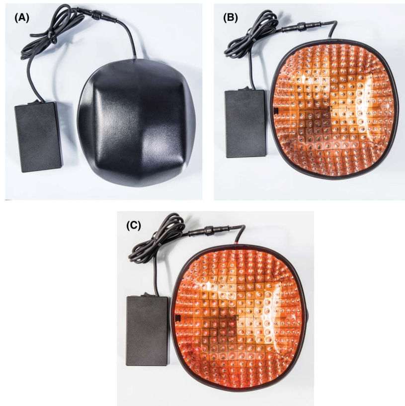
Figure 1. Dome laser device: (A) exterior view of device and controller; (B) interior view of an active unit; and (C) interior view of active device during operation.
